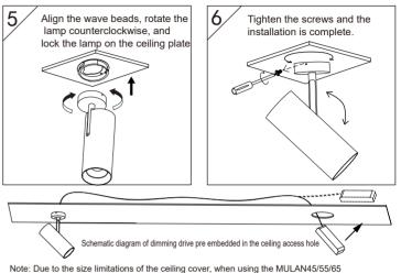
Note: Due to the size limitations of the ceiling cover, when using the MULAN45/55/65 surface-mounted remote dimmable driver, the driver should be pre-embedded in the ceiling access hatch to connect the wires. For the MULAN90 surface-mounted type, the inner hole size of the ceiling cover is large enough, so the driver can be directly inserted through the top of the fixture.
